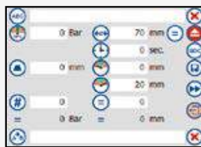
Input of pressure, hold time, opening diameter, preselection counter and press dies (parameter).
