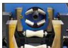
Clamping and guiding unit with wheels for up to 5"-hoses.
