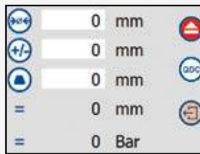
Input of press diameter, correction values and press jaws (automatically).
