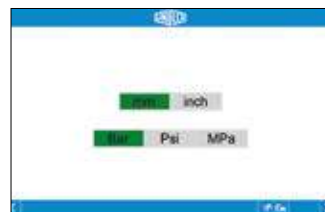
In the green area, the currently set measurement unit is displayed. By tapping a button, the corresponding measurement unit is set.
